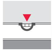
Horizontal **inverted position** (overhead measuring)
